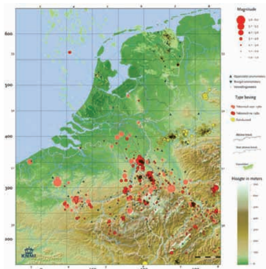
FIG. 1: SEISMICITY IN THE NETHERLANDS AND ITS IMMEDIATE SURROUNDINGS IN THE PERIOD OF 1900–2004. RED CIRCLES INDICATE NATURAL TECTONIC EARTHQUAKES, YELLOW CIRCLES INDUCED EVENTS.
